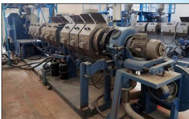
ibility of the devices, which can produce a wide range of polymer shapes, from filaments to blown films, by altering the arrangement of screws and extrusion molds.
